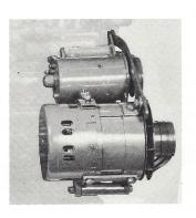
The 100 ampere alternator securely mounted on an extension of the front motor support takes heavy electrical loads in stride.
